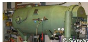
Frankfurt, DE Quasi-Maxwellian neutron generator
